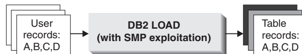
Figure 12. Record Order in the Source Data is Preserved When Intra-partition Parallelism is Exploited During a Load Operation
