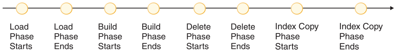
Figure 3. The Four Phases of the Load Process: Load, Build, Delete, and Index Copy
