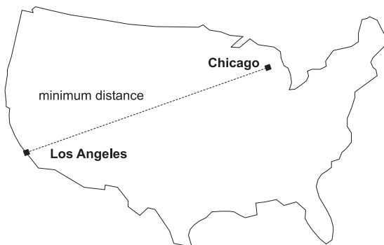
Figure 20. Minimum distance between two cities. ST_Distance can take the coordinates for the locations of Los Angeles and Chicago as input, and return a value denoting the minimum distance between these locations.
