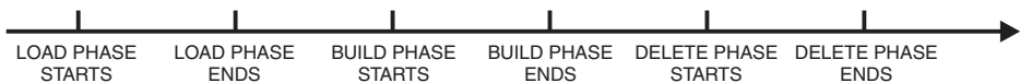
Figure 1. The Three Phases of the Load Process: Load, Build, and Delete. Associated table spaces are in load pending state from the beginning of the load phase until the end of the build phase, and in delete pending state from the end of the build phase until the end of the delete phase.
