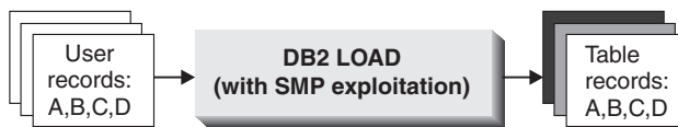
Figure 6. Record Order in the Source Data is Preserved When Intra-partition Parallelism is Exploited During a Load Operation
