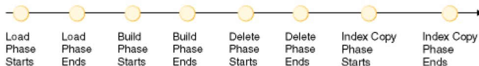
Figure 3. Phases of the Load Process for Row-organized Tables
