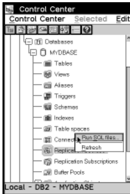
Figure 16. The Run SQL files menu choice. The Run SQL files menu choice is used to run deferred SQL files for the replication object you select.
