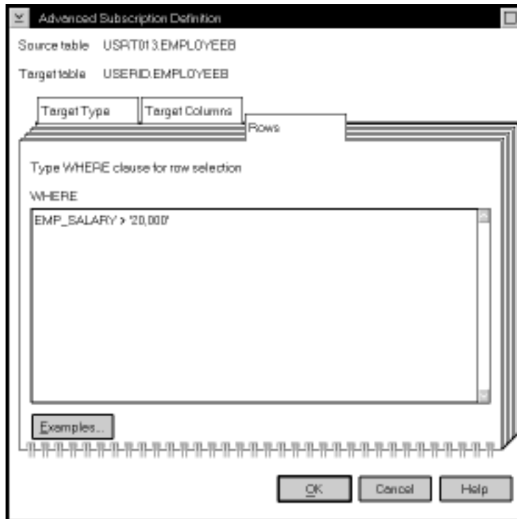
Figure 26. The Rows Page of the Advanced Subscription Definition Notebook. You can subset the rows for the target table by typing in a WHERE clause.
