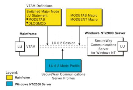
The following image illustrates the interrelationships required when defining the name of the physical unit/control point provided by SecureWay Communications Server for NT:
