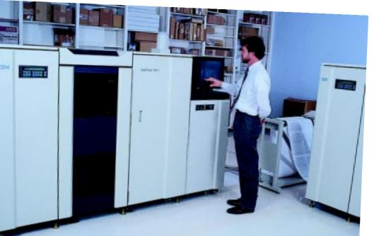
an IBM InfoPrint 60, IBM Print Services Facility (PSF™) for AIX, IBM Printing Systems Manager (PSM) for AIX, IBM EDMSuite OnDemand software and COLD Archival/Retrieval for CD-ROM creation, all attached to an IBM RS/6000™ server.
