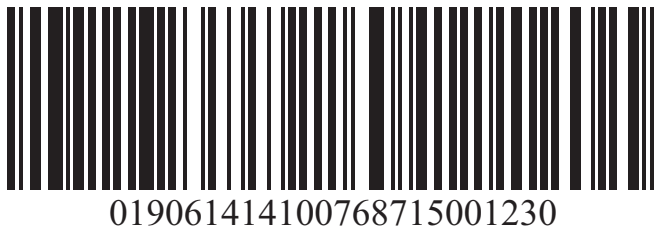
SCC-14 and Sell-By Date Concatenated in a UCC/EAN-128 Symbol (encoding \overset{F}{\underset{I}{\text{019061414100768715001230}}} )
