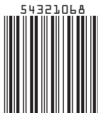
Interleaved 2-of-5 (encoding 54321068)
