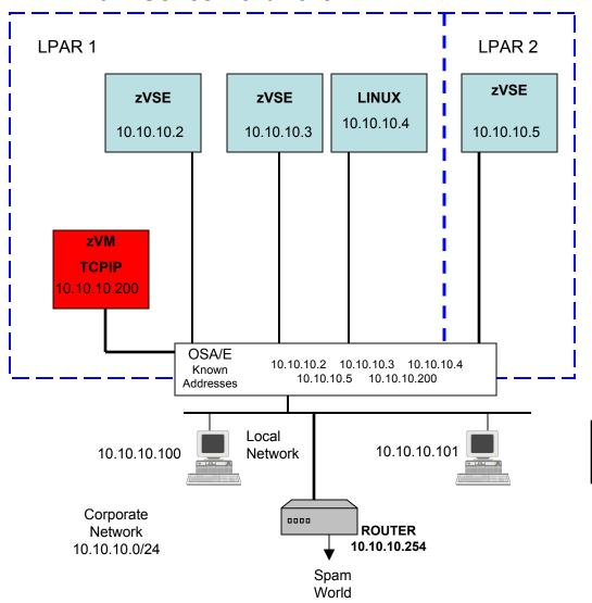
Each VSE/ESA guest is given a set of Sub channel Addresses with which to access the OSA card.
