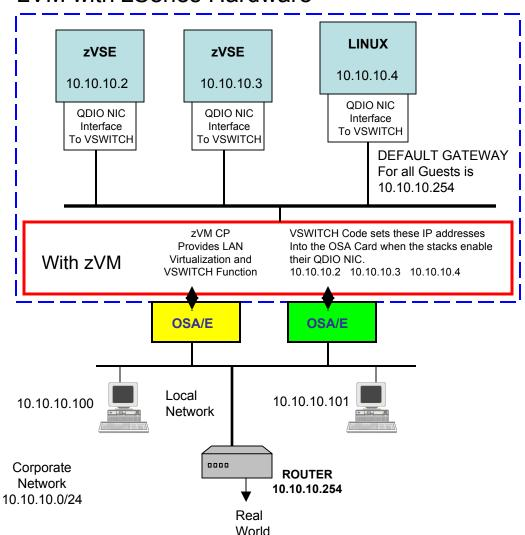
The VSWITCH by its nature provides a "flat network" topology, it acts like an IP bridge between the virtual Network and the corporate network. At zVM5.1 VSWITCH can be a layer 2 or Layer 3 switch.
