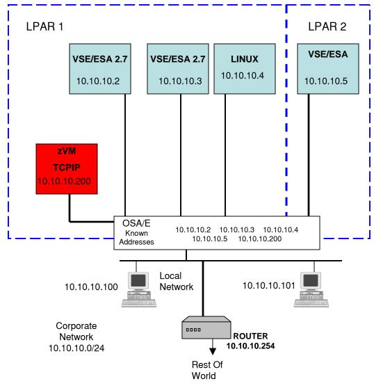
Each VSE/ESA guest is given a set of Sub channel Addresses with which to access the OSA card.
