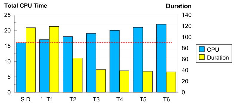
NPS ~ 0.10 -- 9 engines (not characteristic of most real workloads) High CPU intensity, very low I/O content
