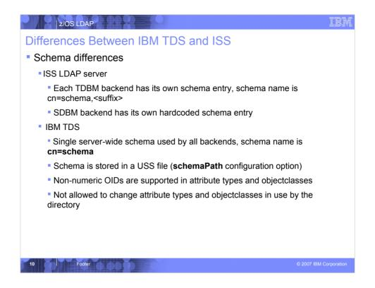
The schema is now named cn=schema. The schema entry is in its own backend and is stored in a file in the Unix System Services file system, with a name of **schema.db**. By default the file is stored in the /var/ldap/schema directory, but the directory can be changed using the **schemaPath** configuration option. The file name cannot be changed. The LDAP server must have read/write access to the schema file and directory.
