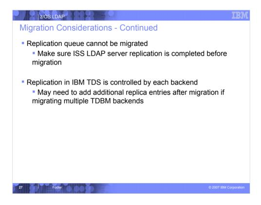
The IBM TDS TDBM backend uses different replication tables than in the ISS LDAP server. The contents of the ISS LDAP server replication tables cannot be migrated. Instead, all replication processing must be completed before migration so that these tables are no longer needed. If replication processing is not completed, then some replicas may be out of synch with the master LDAP server after migration.
