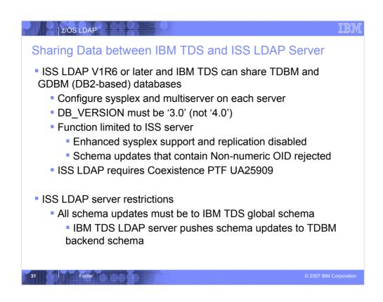
A TDBM database can be shared between an ISS LDAP server and an IBM TDS in a sysplex. The ISS LDAP server must be z/OS V1R6 or later (not V1R5). Each server can read and write TDBM entries. Both servers must be configured in multiserver mode with sysplex support. The database level must be '3.0', which is supported by both servers. The PTF for APAR OA15948 must be applied to the ISS LDAP server to allow it to share TDBM data.
