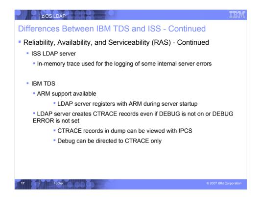
The IBM TDS registers itself with the z/OS Automatic Restart Management (ARM) if the **armName** option is specified in the global section of the configuration file. ARM can be used to react to a failure of the LDAP server.
