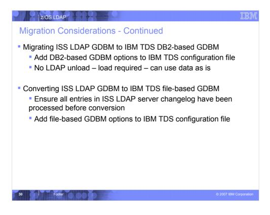
A GDBM backend in an ISS LDAP server can easily be migrated to a DB2-based GDBM backend in an IBM TDS. The only change is to add the backend to the IBM TDS LDAP server configuration file. The GDBM database does not need to be updated to be accessible to the IBM TDS.
