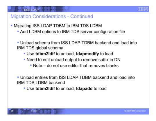
When migrating from a TDBM backend in an ISS LDAP server to an LDBM backend in an IBM TDS, both the TDBM backend schema and the TDBM entries must be unloaded from the ISS LDAP server and then loaded into the IBM TDS. The unloaded schema will start with dn: cn=schema,<suffix>. This must be changed to just dn: cn=schema. Do not use an editor that removes trailing blanks from a line – this could mess up continuation lines in the file and cause load to fail.
