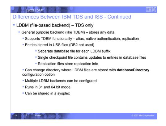
LDBM is a new general purpose backend provided by the IBM TDS. It stores its entries in files within the Unix System Services file system. There are two types of files used by LDBM, database files and the checkpoint file.
