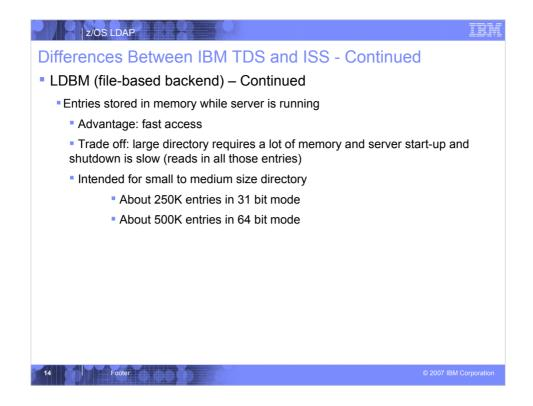
When the IBM TDS is started, all of the LDBM entries are read into memory, providing very fast access to the entries. However, a large LDBM directory will use a lot of memory and can require a long time to initialize when the server is started.
