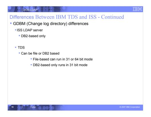
The IBM TDS allows the changelog backend, GDBM, to be configured to store the change log entries in either DB2 or files. The use of the dbuserid option in the GDBM section of the configuration file indicates whether the GDBM backend is DB2-based; otherwise, the GDBM backend is file-based.
