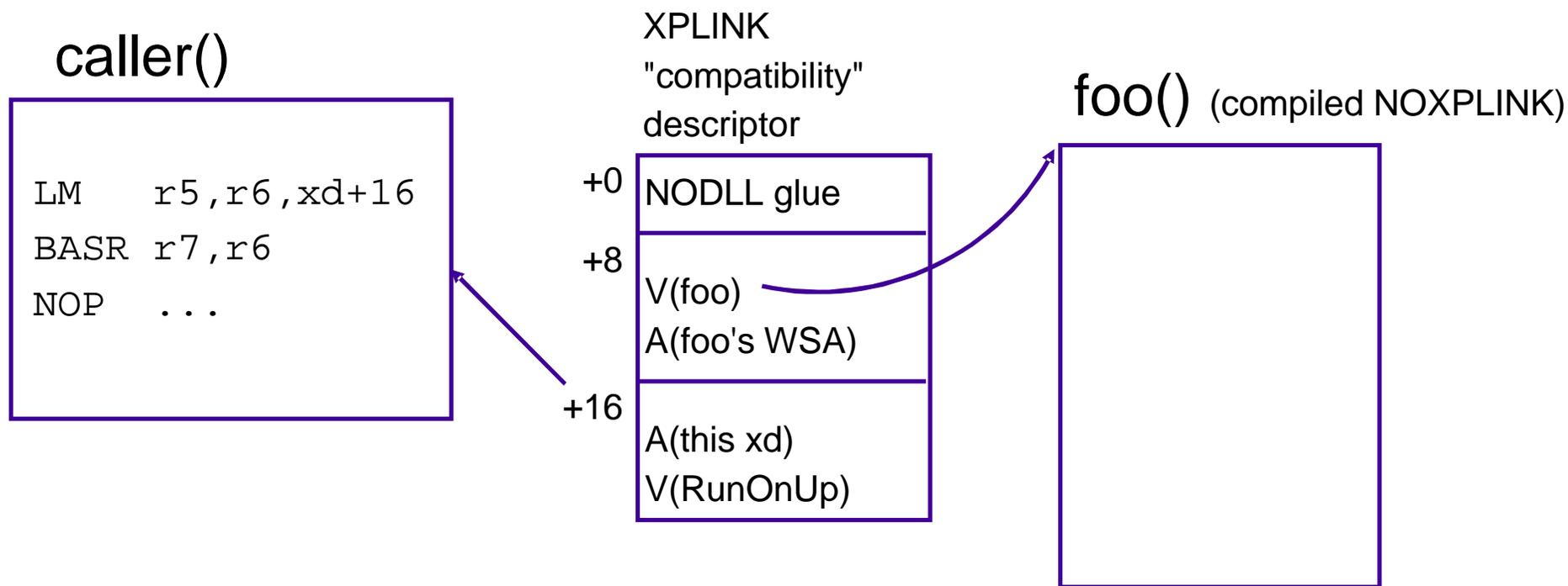
Compatibility between XPLINK and non-XPLINK functions is at the Program Object boundary, and implemented through the glue code.
