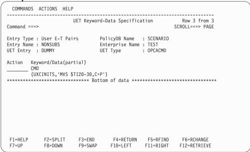
This example shows a command that is not related to a subsystem known to SA z/OS (see "Non-Subsystem Operations" on page 139), and which, accordingly, must be defined as a USER E-T pair (see "Non-Subsystem Operations" on page 139). The jobname of the OPC request would be DUMMY.
