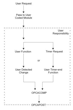
Figure 64. Request Flow for a Subsystem-Related User Function
