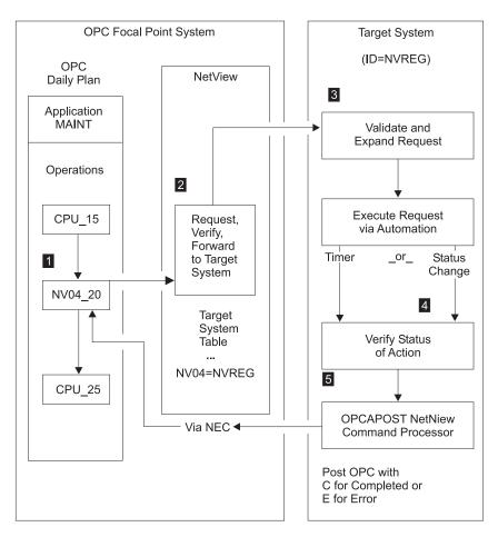
Figure 41. NetView-OPC Interface Flow. Syntax and definition errors, target system availability, recovery, and resynchronization via OPC API and NetView PPI are not shown in this example.
