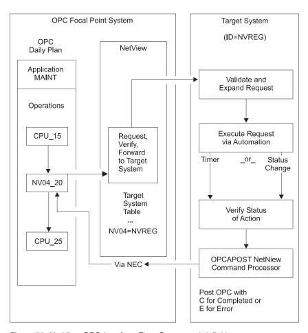
Figure 32. NetView-OPC Interface Flow. Syntax and definition errors, target system availability, recovery, and resynchronization via OPC API and NetView program-to-program interface are not shown in this example.
