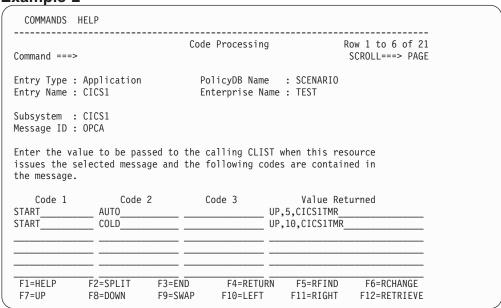
This example shows two entries, one for an automatic start, and one for a cold start, of a subsystem called CICS1. The AUTO or COLD parameter is added to the START request in OPC to indicate which one of several startup procedures is to be used. Presumably the two operations will take differing amounts of time, so the timer intervals are different.
