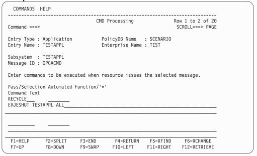
This example shows a RECYCLE type of operation (bring the subsystem down and restart it immediately) being defined. Note that the command to be issued is EVJESHUT, which will issue the
