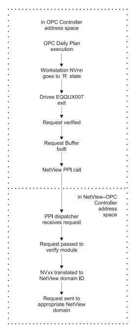
Figure 43. Request Handling in the OPC Controller Processor
