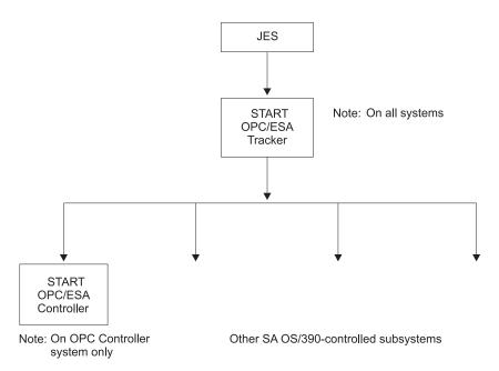
Figure 40. OPC/ESA Startup During IPL Process
