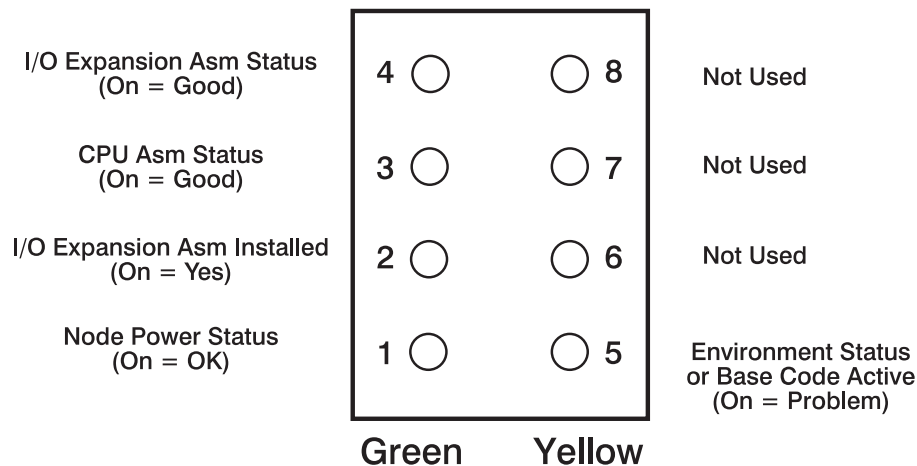
Figure 3-1. 332 MHz SMP and POWER3 SMP Thin and Wide Node LEDs
