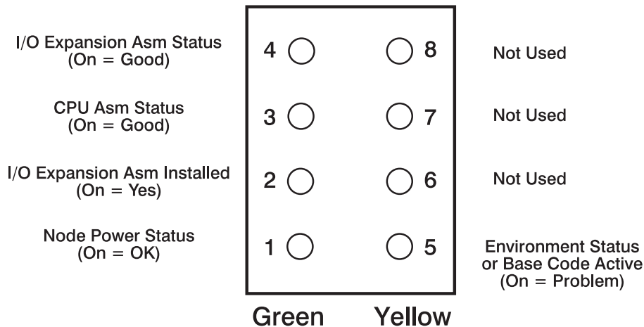
Figure 3-2. 332 MHz SMP and POWER3 SMP Thin and Wide Node LEDs
