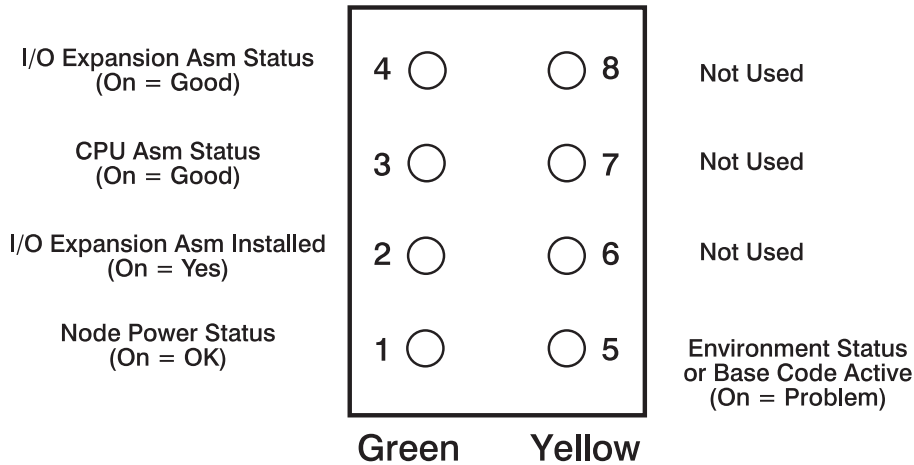
Figure 1-5. 332 MHz SMP Node supervisor card LEDs
