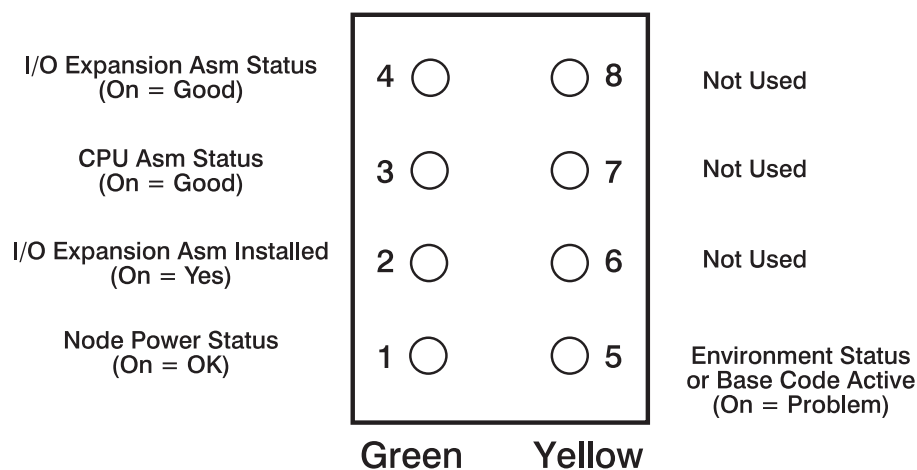
Figure 1-6. POWER3 SMP Thin and Wide Node supervisor card LEDs
