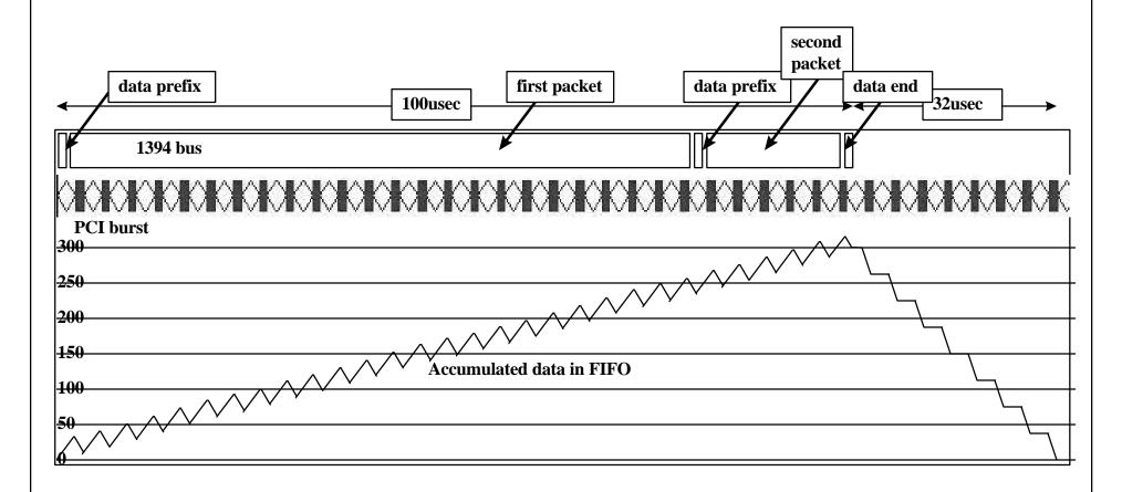
with 2.5usec arbitration latency and burst size of 32
