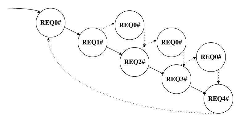
♦ In controlled environment, REQ0# can win every other PCI arbitration. This gives priority to performance-hungry application like 1394 with 50% of total PCI bandwidth
