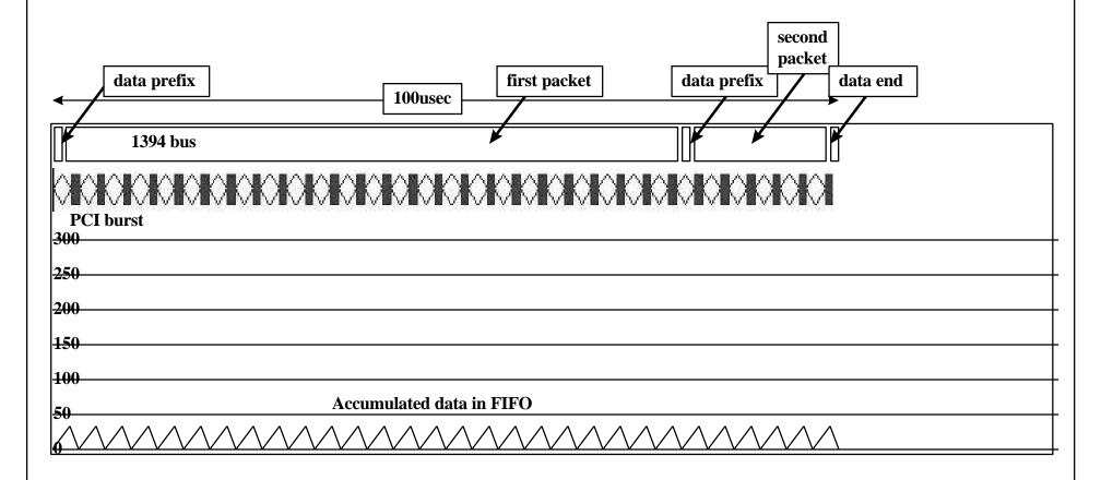
with 1.6usec arbitration latency and burst size of 32
