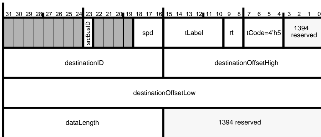
Figure 7-10 — Block read request transmit format
