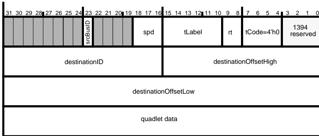
Figure 7-9 — Quadlet write request transmit format
