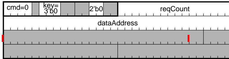
Figure 9-1 — OUTPUT_MORE command descriptor format
