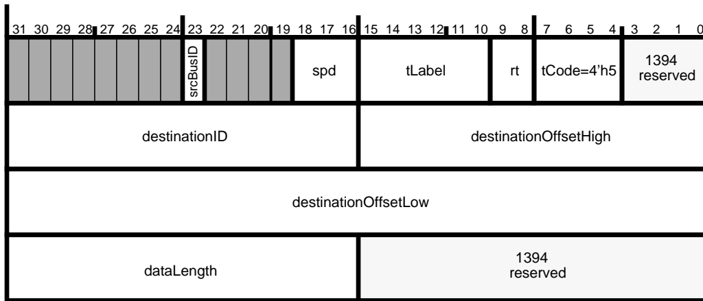
Figure 7-10 — Block read request transmit format
