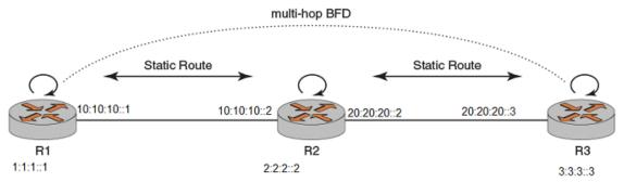
Consider a scenario in which you have three systems, R1, R2, and R3. R1 and R2 share a static route, R2 and R3 also share a static route. The following list provides the addresses of R1, R2, and R3.
