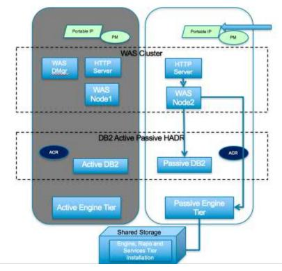
Failure: The machine in dark grey colour has failed all the communication to that machine is stopped.
