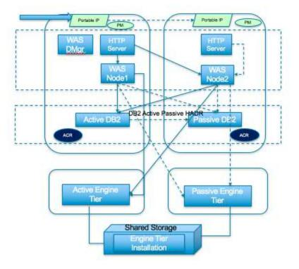
WebSphere Application Server on the passive server machine has a WebSphere node and HTTP Server installed while active server machine also has WebSphere Deployment Manager installed along with these. The HTTP Server takes care of distributing the load between the WebSphere nodes in a round robin fashion.
