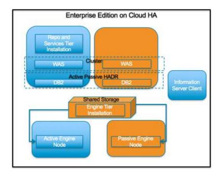
Virtual servers with dedicated CPUs are provided for small and medium plans of IBM Information Server on Cloud Enterprise Edition High Availability. The servers in the large plan are in a bare metal environment. Each of the plans below are given with four server machines.
