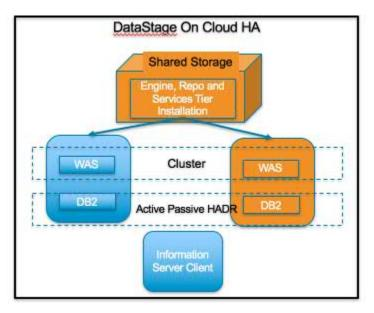
Virtual servers with dedicated CPUs are provided for the small and medium plans of IBM DataStage on Cloud High Availability. The servers in the large plan are bare metal. Both the server machines will have shared file storage along with non-shared storage.
