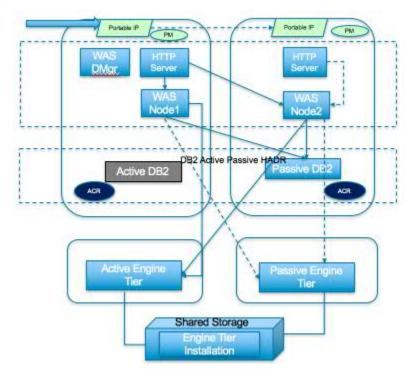
Failure: Active DB2 shown in the dark grey colour goes way, and all database transactions fail.
