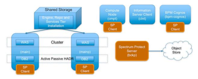
Spectrum Protect server software is installed in the Spectrum Protect server machine and the Spectrum Protect Client software is installed in the rest except the IIS Windows Client machine.
