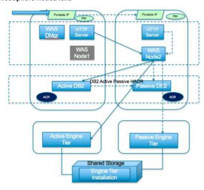
*Failure:* The WebSphere node, Node 1 shown in dark grey colour goes away, and all the connections between this and other processes are broken.
