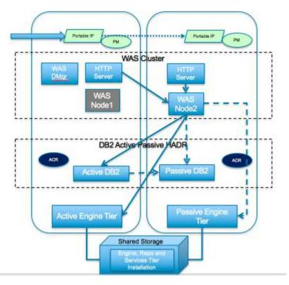
Failure: The WebSphere Application Server node, Node 1 shown in dark grey colour goes away, and all the connections between this and other processes are broken.
