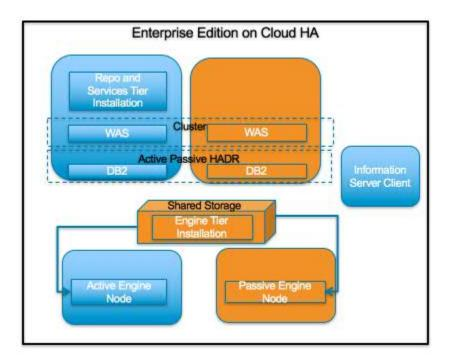
Virtual servers with dedicated CPUs are provided for small and medium plans of IBM Information Server on Cloud Enterprise Edition High Availability. The servers in the large plan are in a bare metal environment. Each of the plans below are given with four server machines.
