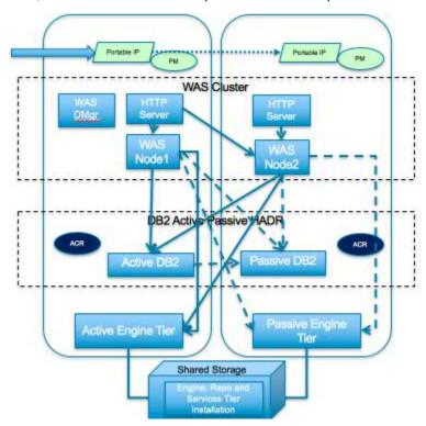
WebSphere Application Server on the passive server machine has a WebSphere node and HTTP Server installed while active server machine also has Deployment Manager installed along with these. HTTP Server takes care of distributing the load between the WebSphere Application Server nodes in a round robin fashion.
