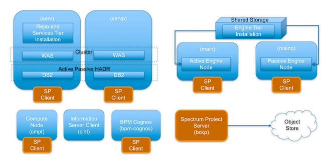
Spectrum Protect server software is installed in the Spectrum Protect server machine and the Spectrum Protect Client software is installed in the rest except the IIS Windows Client machine.
