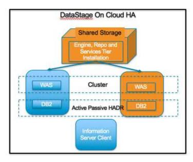
Virtual servers with dedicated CPUs are provided for the small and medium plans of IBM DataStage on Cloud High Availability. The servers in the large plan are bare metal. Both the server machines will have shared file storage along with non-shared storage.
