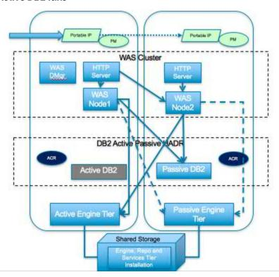
Failure: Active DB2 shown in the dark grey colour goes away, and all database transactions fail.
