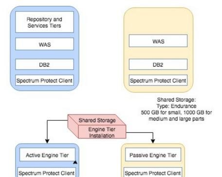
Two Server machines each with Spec: OS Version: RHEL 7.4 Maipo 4 core and 16 GB RAM for small parts 8 core and 32 GB RAM for medium parts 8 core and 32 GB RAM for large parts Server Type: Virtual Server for small and medium, Baremetal for large
