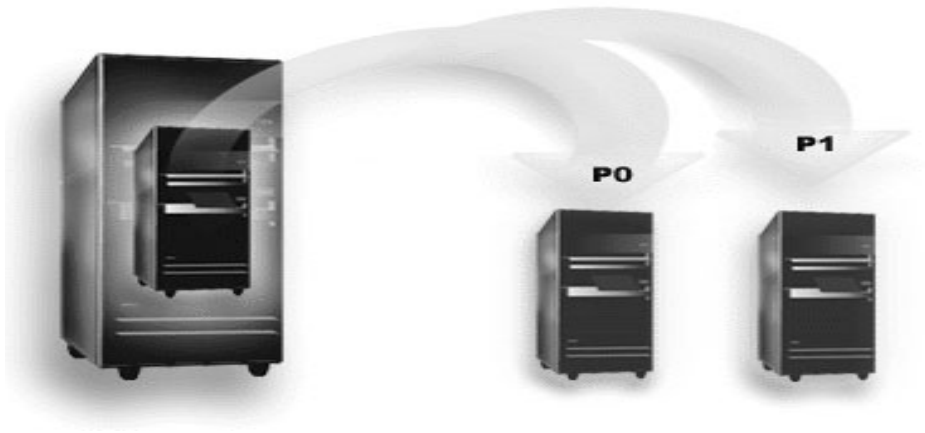
Figure 4.1 LPAR Logical View - one server looks like multiple servers
