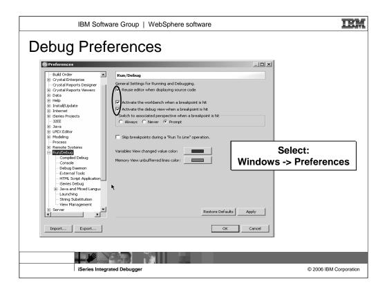
When using the debug editor, check the 'Reuse editor when debugging source code' check box if you want only one tab for multiple source in the debug editor. Switching to a different source can then be done from the call stack or the Programs view. If de-selected, each source will have its own tab and selecting its tab will display the source.
