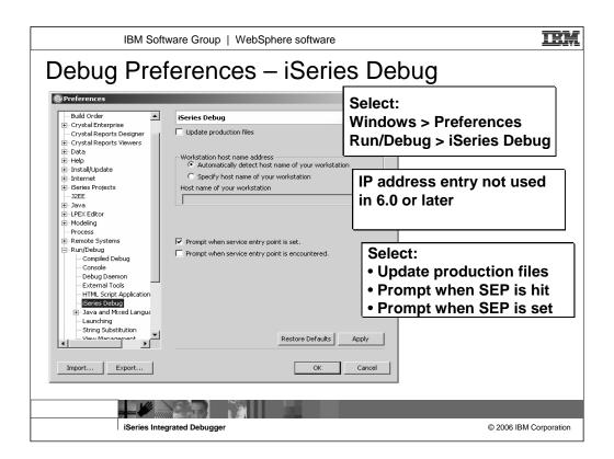
By default, Update production files is not selected. Check the check box to allow the debugger to update production files. You need to set this preference if you are using service entry points to start your debug session and want to be allow update production files.
