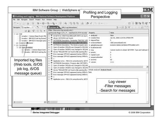
The Profiling and Logging perspective allows you to import i5/OS logs and message queues.
