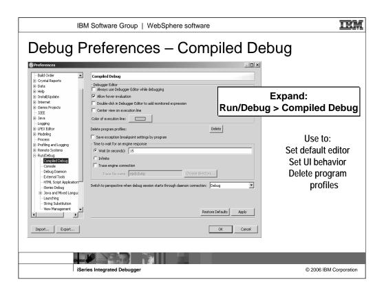
Un-checking the 'Always use Debugger Editor while debugging' check-box will use the LPEX editor to display the source while debugging.
