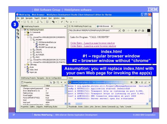
This is the index.html page that was generated based on your choices during conversion or by settings in the Properties dialog. If you click on a link, the WebFacing run-time servlet will be invoked (in WFRun.jar). Passed as a parameter is the invocation file that contains the system name and the name of the program to call. To see how WebFacing is invoked choose View/Source from the browser window.
