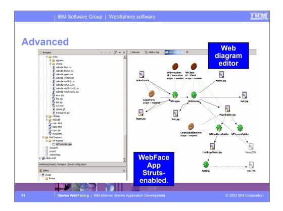
When you enable Struts support, you can develop Struts-based WebFacing services with the Struts builder, a visual development environment for building Struts services. Using the builder, you can drag and drop JSPs, action mappings, form beans, and Java beans onto a Web diagram. In the diagram, you make connections between items on the palette, and then activate those items by double-clicking and editing them through a wizard or source code.
