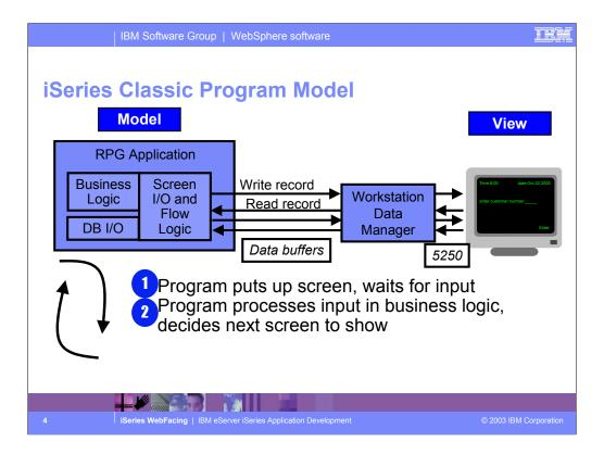
In the green-screen environment, the application performs READs and WRITEs to the workstation. The application data is sent to Workstation Data Manager. The Workstation Data Manager merges application data with the display file. The Workstation Data Manager generates a 5250 datastream that is sent to the display.
