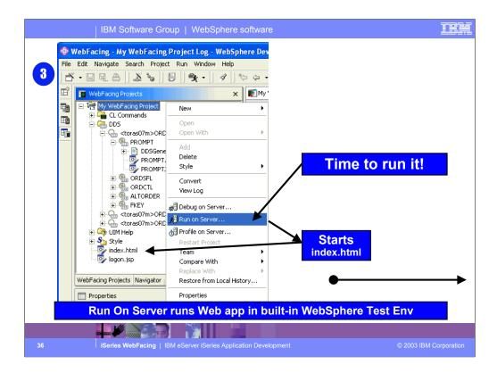
Once the application has been converted it can be tested in the built-in WebSphere Test Environment. Locate the index.html page and choose Run on server. If not yet started, the WebSphere Test Environment will start. The index page will appear in the internal browser view.
