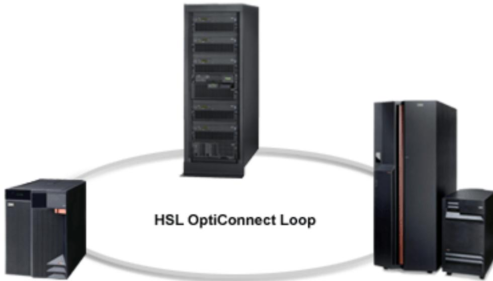
Figure 2. Three-system HSL OptiConnect loop
