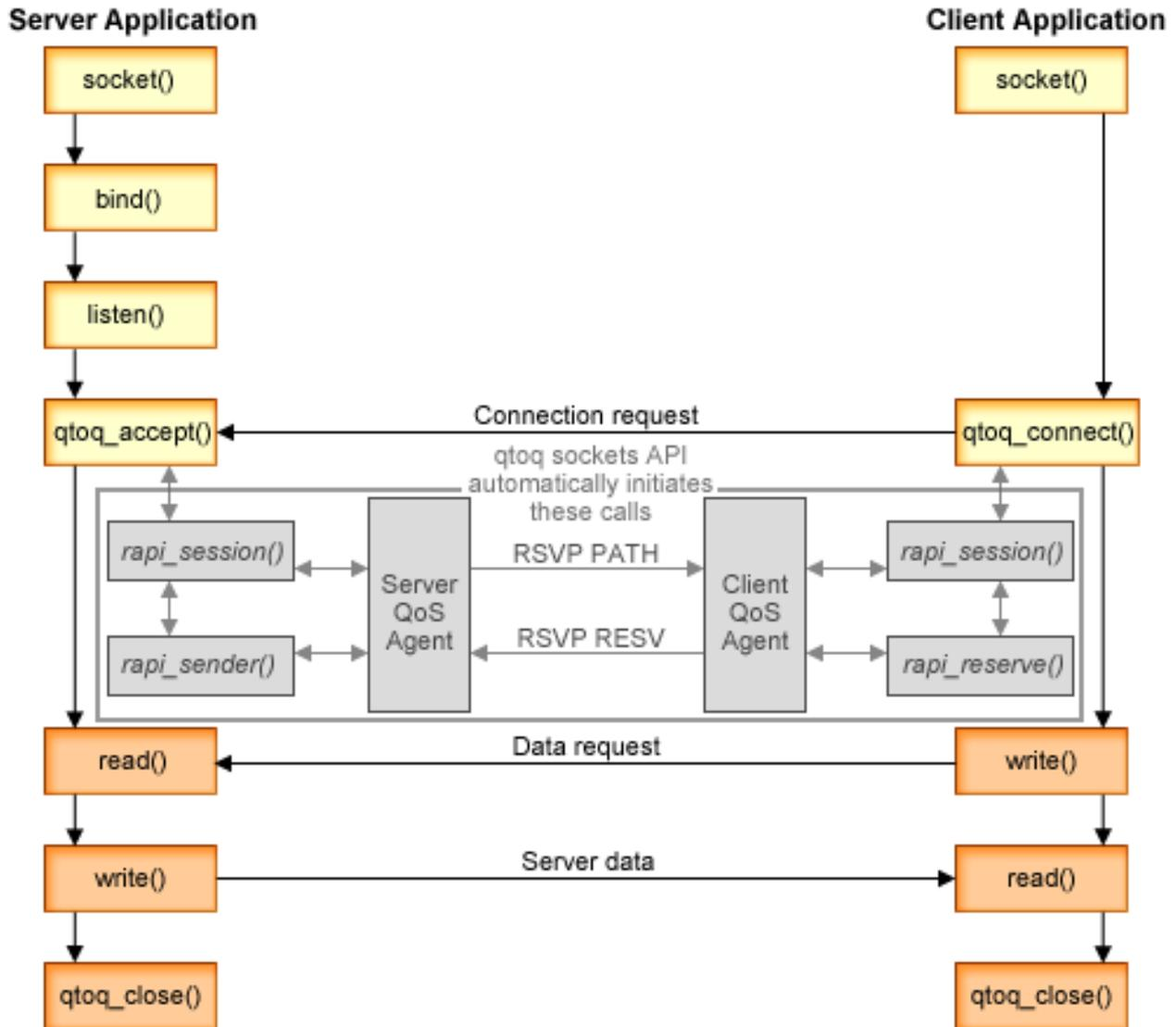
**qtoq flow of events:** The following sequence of socket calls provides a description of the figure. It also describes the relationship between the server and client application in a connection-oriented design. These are modifications of the basic socket APIs.
