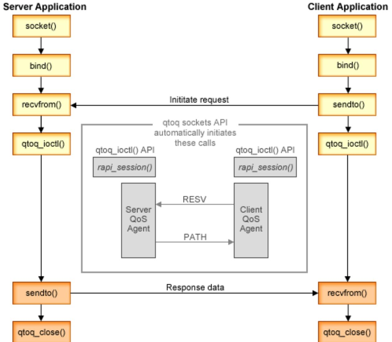
**qtoq flow of events:** The following sequence of socket calls provides a description of the figure. It also describes the relationship between the server and client application in a connectionless design. These are modifications of the basic socket APIs.
