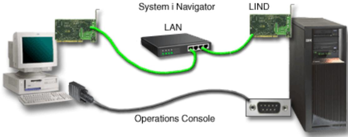
Figure 2. System i Navigator and Operations Console configuration over separate connectivity
