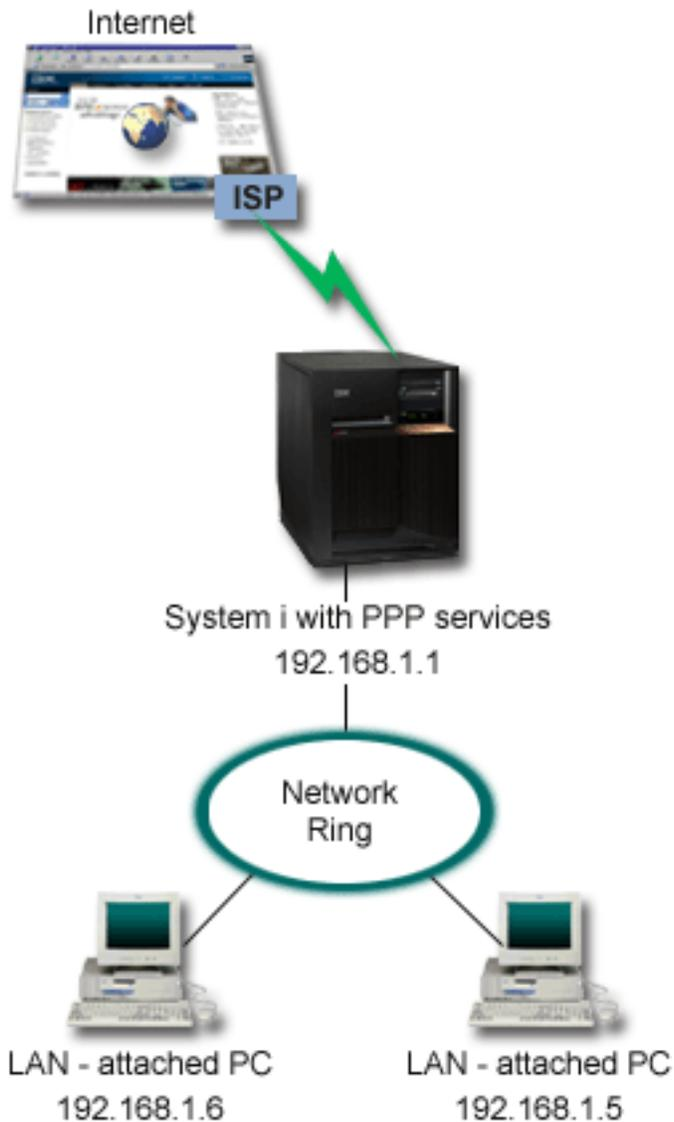
Figure 5. Connecting your office LAN to the Internet with a modem
