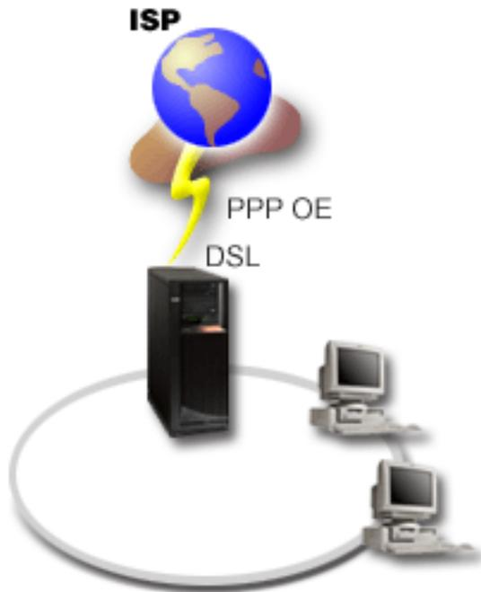
Figure 3. Connecting your system to an ISP with PPPoE
