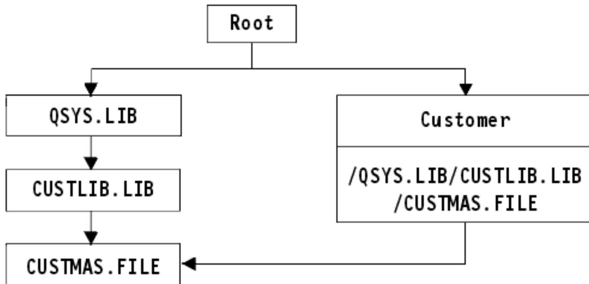
Figure 4. An Object with a Symbolic Link—Example
