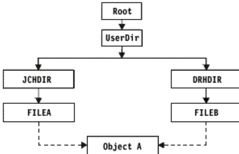
Figure 3. An Object with Hard Links—Example
