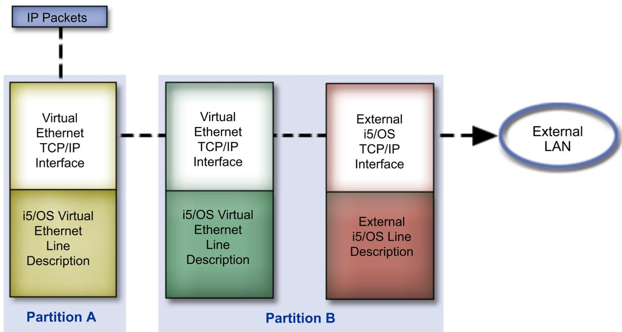
IP traffic initiated by partition A goes from its own virtual Ethernet interface to the virtual Ethernet interface on partition B. By implementing TCP/IP techniques used to connect virtual Ethernet to external LANs, you can enable the IP packets to continue on to the external interface and toward their destination.
