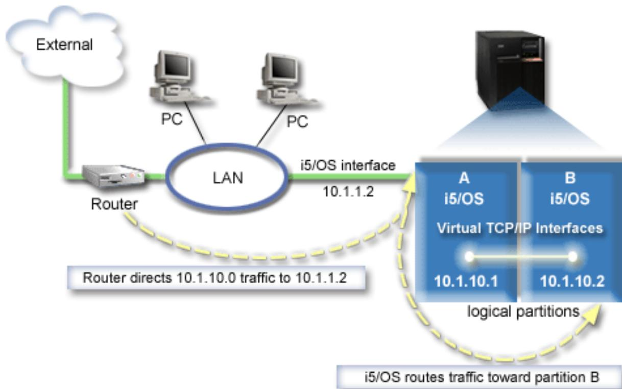
The existing TCP/IP interface (10.1.1.2) connects to the LAN. The LAN is connected to remote networks with a router. The virtual TCP/IP interface on partition B is addressed as 10.1.10.2 and the virtual TCP/IP interface on partition A as 10.1.10.1. In i5/OS, if you turn on IP datagram forwarding, i5/OS will route the IP packets to and from partition B. When you define your TCP/IP connection for partition B, the router address must be 10.1.10.1.
