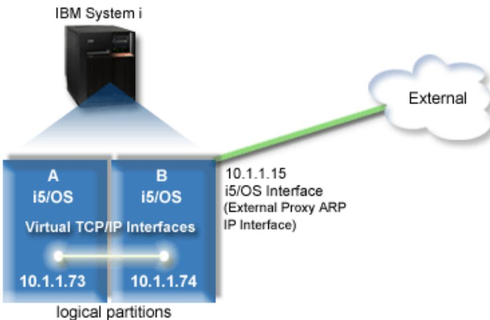
In this example, TCP/IP traffic from partition A runs across the virtual Ethernet to the 10.1.1.74 interface on partition B. Because 10.1.1.74 is associated with the external proxy ARP interface 10.1.1.15, the packets continue out of the virtual Ethernet using the proxy ARP interface.
