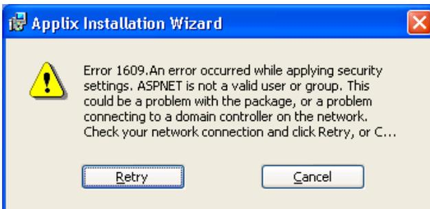
You must define the ASPNET user before installing TM1 Web. To create the ASPNET user:
